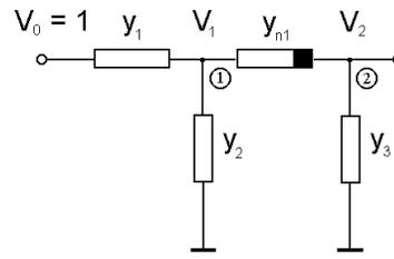
Fig. 1 Two-node nonlinear passive network
