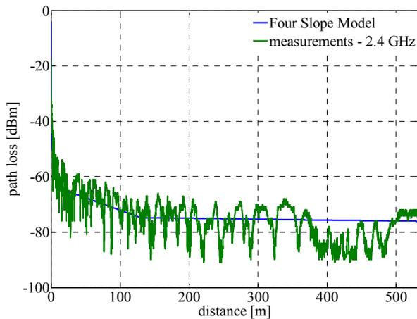
Fig. 9. Comparison of measurement results and path loss model for tunnel;  $f= 2.4$  GHz
